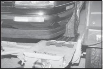
**Step 4.** Before loading (and unloading) towed vehicle make sure platform and towed vehicle are in straight alignment. Tow dolly must be completely and properly hooked up to the towing vehicle. **Towing vehicle must be larger and at least 1000 lbs. heavier than the tow dolly and towed vehicle combined.**
